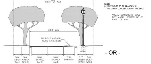
2. STREET LIGHTS SHALL BE PELCO POST TOP LUMINAIRE POLES WITH BRISTOL SERIES, DARK SKY LED LUMINAIRES, HOLOPHANE WASHINGTON UTILITY LED LUMINAIRE WITH FLUTED POSTS AND HAMILTON BASES, OR STAFF APPROVED EQUAL, SPACED A MAXIMUM OF 200 FEET AND AT INTERSECTIONS. POLES AND LUMINAIRES SHALL BE POWDER COATED BRONZE FEDERAL STANDARD COLOR 20062. DIRECT BURIAL POLES NOT ALLOWED. SEE WEBSITE FOR DETAILED SPECIFICATIONS.
