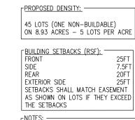
1) NO LOTS MAY HAVE ACCESS ONTO OLD WIRE ROAD. 2) NO FENCES SHALL BE CONSTRUCTED N DRAINAGE EASEMENTS. 3) HEIGHT LIMIT, 35' IF SIDE YARDS ARE 15' OR LESS. 45' IF SIDE YARDS ARE GREATER THAN 15'. 4) DEVELOPER TO CONSTRUCT ALL ADA RAMPS AND SIDEWALKS ALONG COMMON PROPERTY. 5) STREETLIGHTS TO BE PROVIDED BY THE UTILITY COMPANY SERVING THIS AREA.
